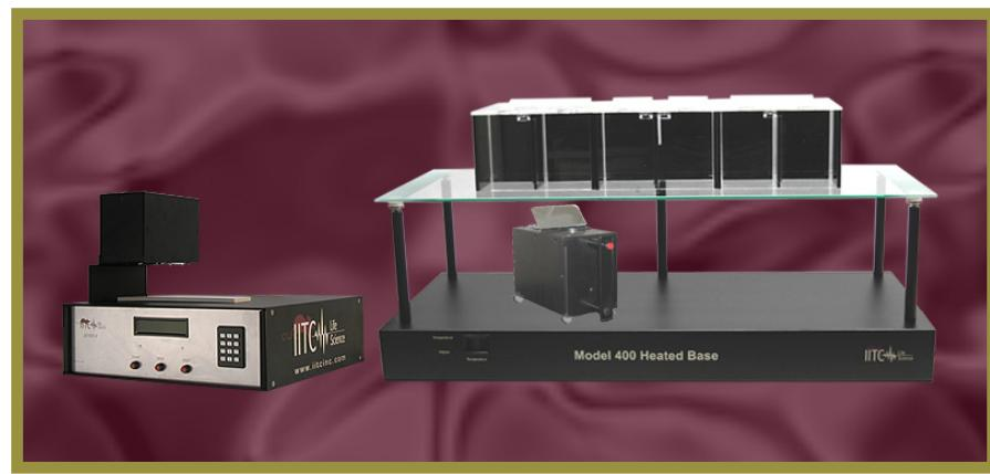
In tail flick mode the test head is attached to the electronics and the heat source sits over a tail groove that has a sensor that detects when the animal flicks its tail. System records and displays time and temperature of test. A humane cutoff timer that can be set by user, will prevent tail tissue damage if test subject does not react within preset time.
